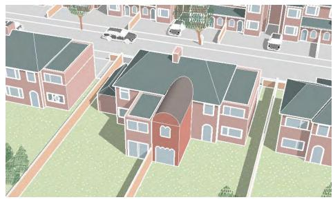
Figure 4.16d: A two-storey extension proposed to a semi-detached house where a neighbour already has a two-storey extension.
