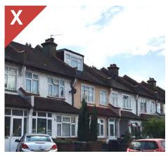
Figure 4.21f: Example of an inappropriate addition of a front dormer to a mid-terrace house. This addition lacks design merit and breaks the uniformity of the roofs that contributes to the positive characteristics of the street.
