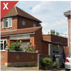
Figure 4.15b: A side and front extension with a series of different roof forms results in a poorly considered composition that has a negative impact on the streetscene.
