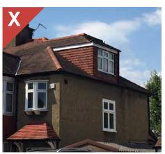
Figure 4.21e: Example of where a side roof extension to a house has not been setback from the original roof. In this situation it has compromised the symmetrical form of the original semi-detached houses and therefore negatively impacts the appearance of street.
