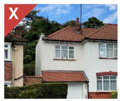
Figure 4.24c: The combination of a pitched roof with a parapet results in an unattractive appearance.
