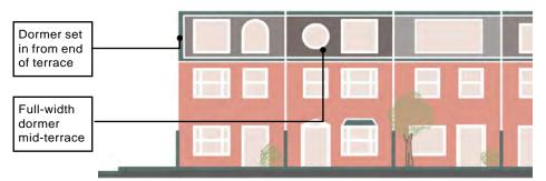
Figure 4.21b: Dormers on a terraced houses that are full-width for midterrace houses, but set in from the edge of a gable end (or hipped roof) on the end of terrace house.
